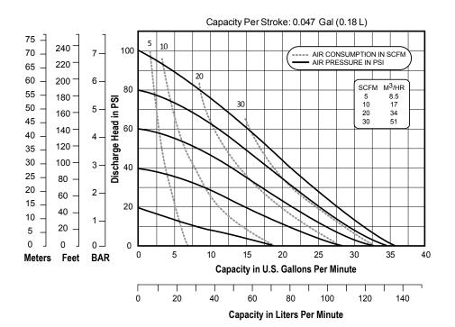
NOTE: Performance based on the following: PTFE fitted pump, flooded suction, water at ambient conditions. The use of other materials and varying hydraulic conditions may result in deviations in excess of 5%.
