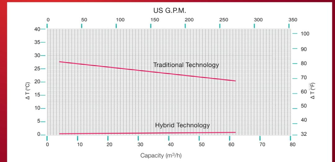
Hybrid technology reduces greatly heat generation in the rear casing region. This benefit is particularly important when pumping low boiling liquids.
