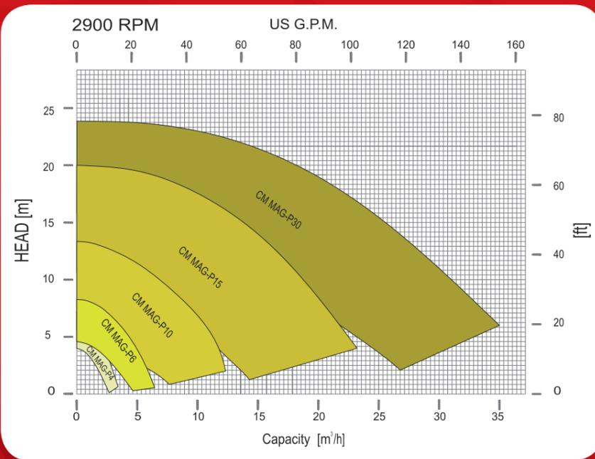
Pump construction and Operative Limits
